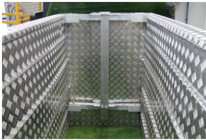
Showing spreader bars
